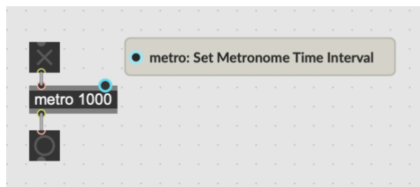
Figure 4.1: Basic metro construction
